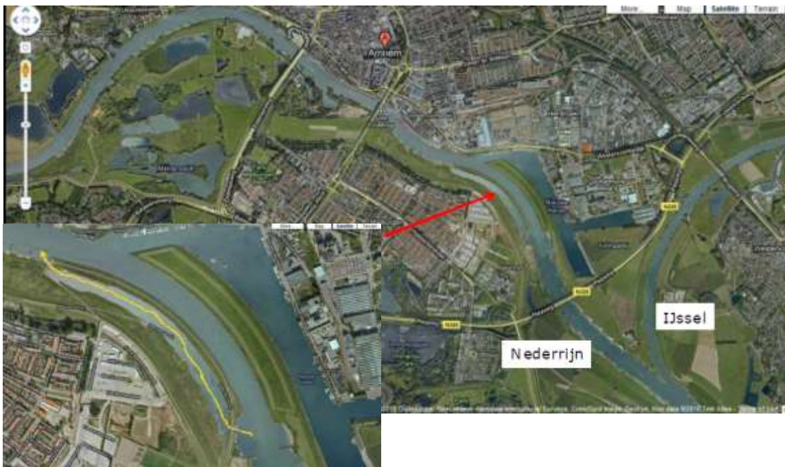
Figure 4 – The construction of a side channel at the Bakenhof site allows natural processes to help form the development of the river and floodplain in this reach of the River Nederrijn.
