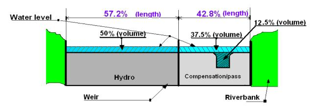
Typical abstraction Weir with a 12.5% or 50% (whichever is greater) compensation requirement elevation at annual average flow
